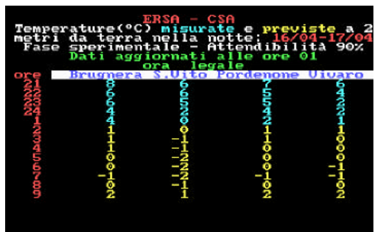
Fig 2. Example of Angela's forecast on a teletext page. Blue figures are the in situ measured temperatures, the yellow ones are the Angela's forecasts
